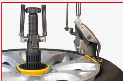
Top bead demounting procedure
