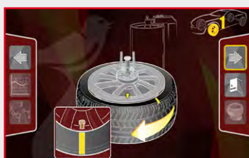
Match-Mounting procedure (rim-tyre)
